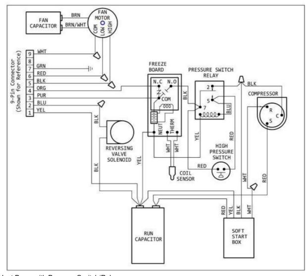
Heat Pump with Pressure Sw itch/Relay
