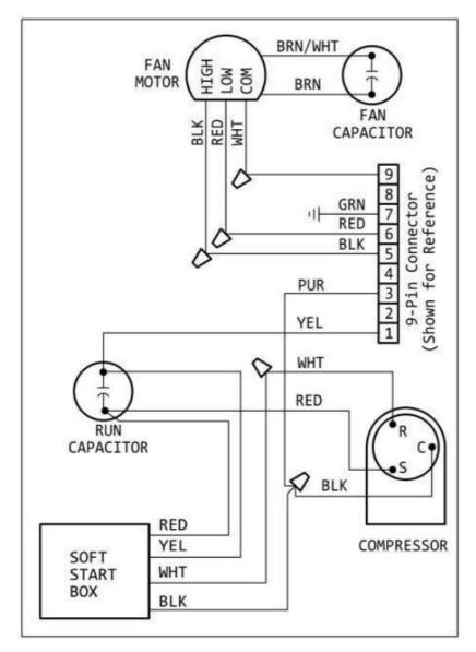
• Air Conditioning Without High Pressure Switch/Relay
