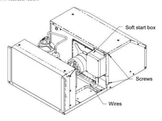
3. Connect with the wire according the diagram of different air conditioner type.
