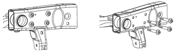
5. Install the supplied Rusty's JL Front Track Bar Frame Brace over the factory track bar mount and align the upper four mounng holes with the four steering box bolt hole locaons and reinstall the factory hard- ware to secure the steering box and brace. Apply Blue Locte to threads before reinstalling these bolts.
