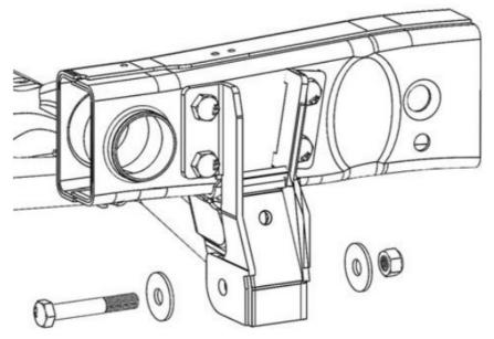
7. Install the supplied (Qty:1) 7/16"-14 x 1-1/4" Length Grade 8 Hex Head Cap Screw, (Qty:2) 7/16" SAE Flat Washer, and (Qty:1) 7/16"- 14 Grade 8 Hex Lock Nut to the hole locaon in the image below. (Note: Do not fully ghten hardware at this **me.**)
