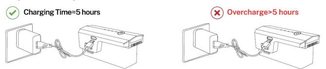
• DO NOT charge the battery immediately after the flight as the temperature may be too high. Wait until it cools down to room temperature before charging again. Due to the battery current output, slight hotness is normal while flying.
