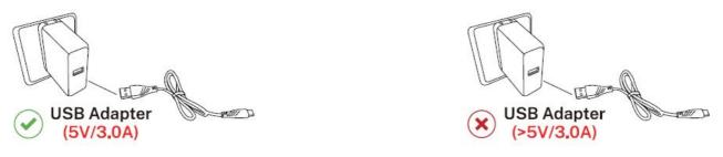
• It is prohibited to use computer USB, simple USB, and inferior charging cables for charging.
