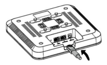
3. Align the square feet on the rear of the AP over the mounting holes on the bracket. Slide the AP into the holes until it clicks into place, as shown in Figure 3-3. Figure 3-3 Fastening the AP
