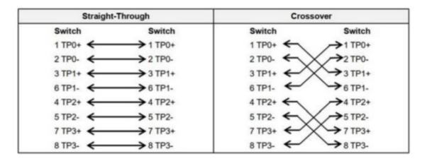
10BASE-T uses Category 3, 4, 5 100-ohm UTP/STP and 1000BASE-T uses Category 5 100-ohm UTP/STP for connections. Both support a maximum length of 100 meters. Table A-1 shows 100BASE-TX/10BASE-T pin assignments.
