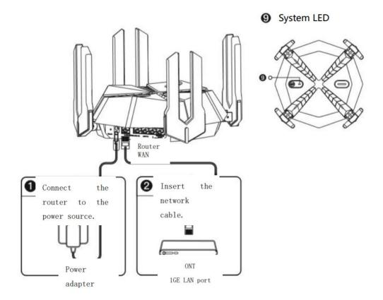
After the system LED is steady on or blinks slowly, connect the router to the default SSID broadcast by the router: @Ruijie-sXXXX. The configuration page will pop up. Then, complete the settings as prompted.
