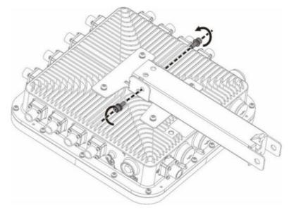
3. Mount the device with the installation pole installed to the fixed support. Use hooks on the installation pole to connect with the support, and tighten a M8 combined screw on the left and right sides.
