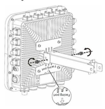
Figure 3-6 Connecting the Mounting Bracket and Installation Pole Based on the Ceiling-mounted Direction
