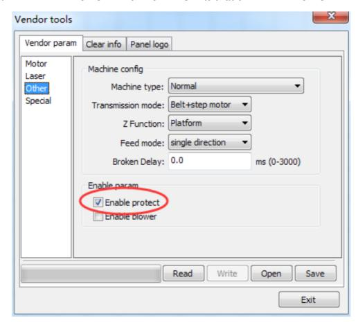
MetalCut → VENDOR SETTING → SPECIAL → (the password is rdtsmm) → height controller type(common) → check follow up(use trigger) → check follow(use trigger). Shown as following:
