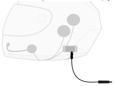
Tuck any excess cabling behind the helmet liner to clean up your installation.
