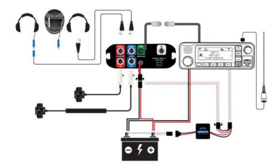
If using optional Active Filter, connect radio and intercom power leads directly to Audio Filter and NOT to the battery.
