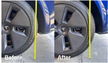
Ground clearance before installation – 23.5" to reference line. After installed the UCSBM1,2, and 3 assembly, the ground clearance increased 0.5".
