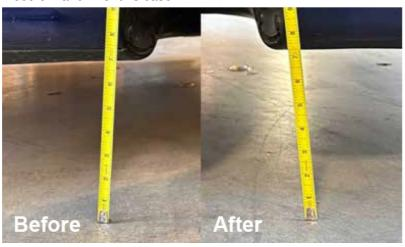
Before installing the from buffer, the ground clearance is 7". Ground clearance after installed UCSBH1 and UCSBH4 – 0.5" increased
