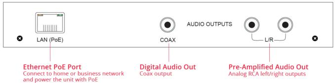
The MS-1 back panel features a stereo RCA output, a digital coax output, an Ethernet PoE port for connecting to the network and for powering the unit. Up to 4 MS-1 stremers can be rack mounted with the optional Rack Mount Kit RM-4VIP2 (2 RU).
