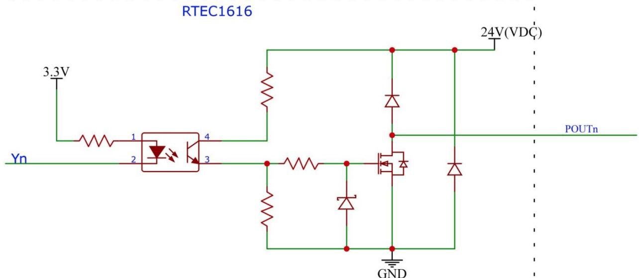
The output port of each channel can output a maximum of 500mA current, and a larger current output can be achieved by connecting multiple output ports in parallel. There is a built-in absorption diode inside the module, which can drive inductive loads.
