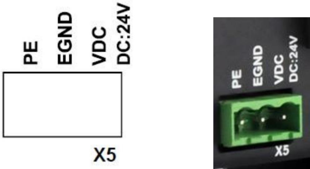
The power interface X5 includes 3PIN terminals, which are defined as follows:
