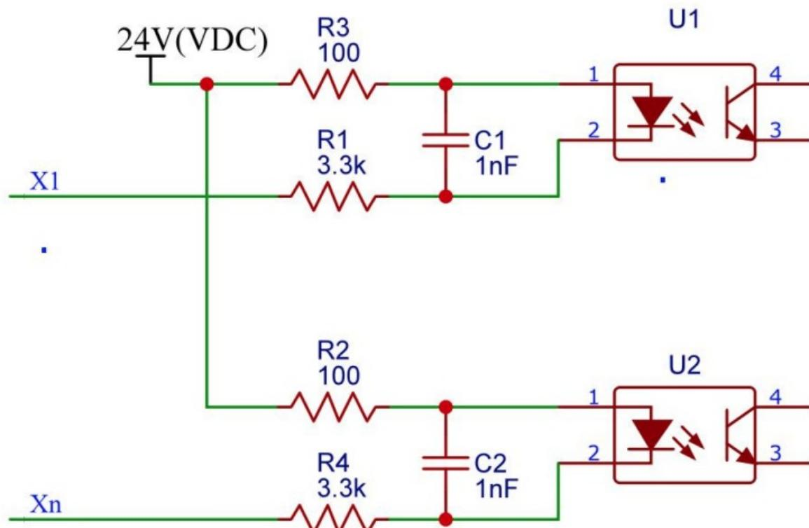
When the external input signal interface type is NPN, the wiring is as follows:
