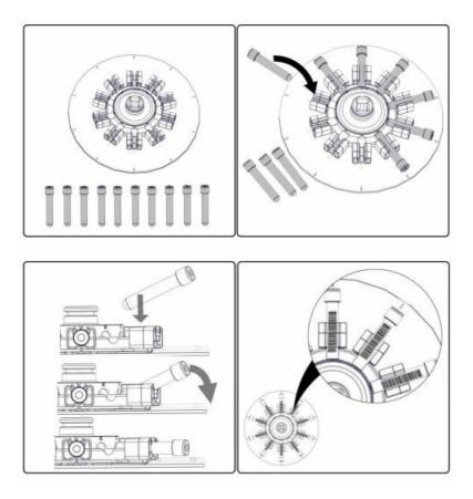
3. Place the rotor back in the instrument. (This is only possible if the needle service cover is closed.)
