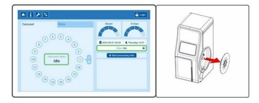
2. Remove already processed tubes from rotor and place new sample tubes with barcodes visible at the front: with a tilting movement and bottom first to prevent damage to the barcode label.
