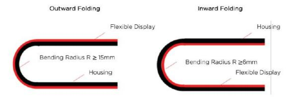
The thickness of the Royole flexible display is only about 0.01 mm, and the bending radius can reach 1 mm. Taking into account the actual use of the development and application, the corresponding cover and laminate have been added to the original flexible display. Therefore, the bending radius of the fully flexible display in the flexible development kit is 15 mm to meet the needs of different usage scenarios. If you have a customized
