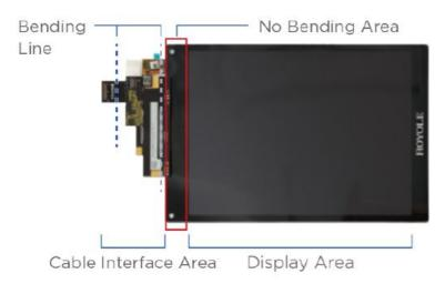
DO NOT bend the line interface area, otherwise it will cause damage to the line/device and cause malfunction.
