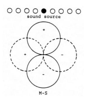
With the SF-24's logo facing the center of the performance, the mic is positioned for X-Y recording. Rotating the SF-24 counter-clockwise by 451/4 positions it for M-S recording. By inserting your SF-24 with the logo in the left slot
