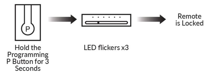
To unlock the remote and allow programming once again, repeat the steps above. For further operations please refer to the motor pairing instructions.
