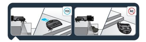
The robot has anti-drop sensors to detect stairs. The robot will change direction when detecting them. For optimum anti-drop sensor efficiency, remove any item (ex: shoe) from the stairs. When using the robot in a raised area, place a physical barrier at the edge of a drop to prevent accidental falls.
