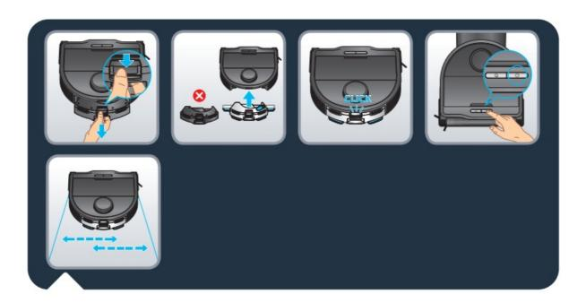
• Unclip the "vacuum only" module by pressing the latch and pull to remove the "vacuum only" module. Take the
