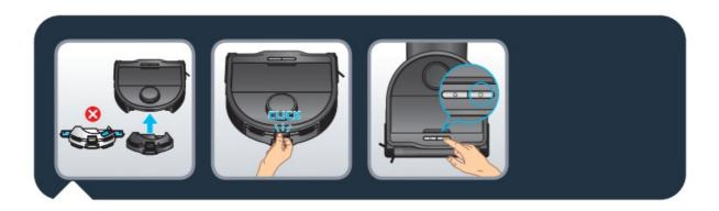
To use the robot without the mopping function ("vacuum only" mode), install the "vacuum only" module at the back of the robot. The module is correctly installed when you hear a « click » sound. Press the « Start » button or use the app to start cleaning. Keep the "vacuum only" module installed in the robot when you don't use the mopping function. The "vacuum only" module is equipped with charging contacts to allow the robot to dock to the station and to charge its battery.
