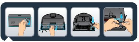
Remove all protections (protective films) on the station and the robot. Reverse the robot, and install the side brush by gently clipping it. The side brush is correctly installed when you hear a clicking sound.
