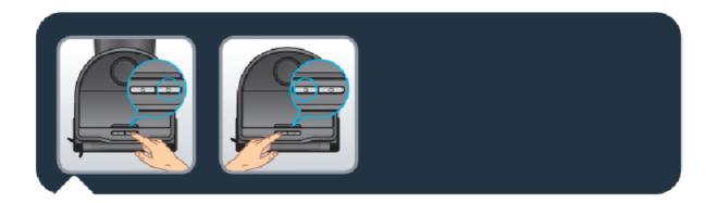
• Press the button « Start » to start automatic cleaning. The robot will scan the area. It will automatically split the room into small zones, first cleans inside the zone in a zig zag, and then cleans zone edges. The robot will
