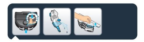
• At the end of the cleaning session, unclip the water tank by pressing the latch and pull to remove the water
