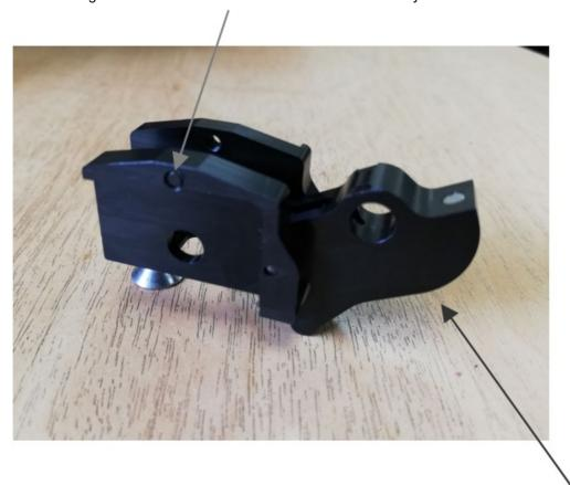
4. The loader is now ready for use.(A grub screw on top of the arm can adjust the amount of grip on the pellet).
