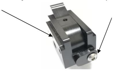
3. On the underside of the loader are location pins.
