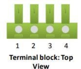
The sensors usually have two pairs of wires of the same color. Connect One pair of the same color wires (say Red) to pins 1 and 2 and the other pair of same color wires (say black) to pins 3 and 4.
