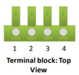
Connect one wire to pin 1 and the other wire to pin 4. Connect a jumper wire between pins 1 and 2 and also between pins 3 and 4 as shown above. For more information on the various configurations of the RTD, please visit the Conax website at
