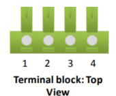
Connect one pair of the same color wires to pins 1 and 2. Connect the other wire to pin 3. Connect a jumper wire between pins 3 and 4.
