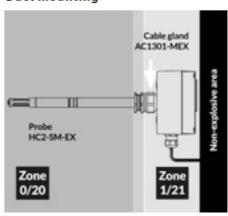
Wall mounting with screw-in sensor
