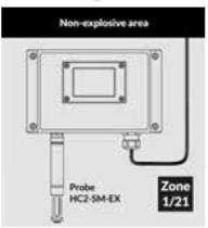
Wall mounting with cable sensor
