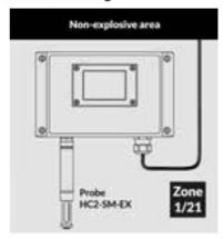
Wall mounting with cable sensor
