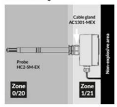
Wall mounting with screw-in sensor
