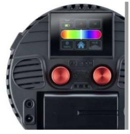
Power off the light and insert the USB stick. Whilst clicking and holding down both knobs, power on the unit. Release knobs when the bootloader dialogue box appears. Select 'YES' to install the firmware. DO NOT power off the light during a firmware update and ensure the update is allowed to complete. A progress bar will appear and upon completion the light will restart.
