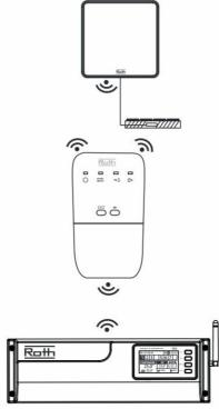
Press the registration button (E) on the Repeater. The registration indicator "out" (D) will now be permantly on and the registration indicator "in" (C) will start flashing.
