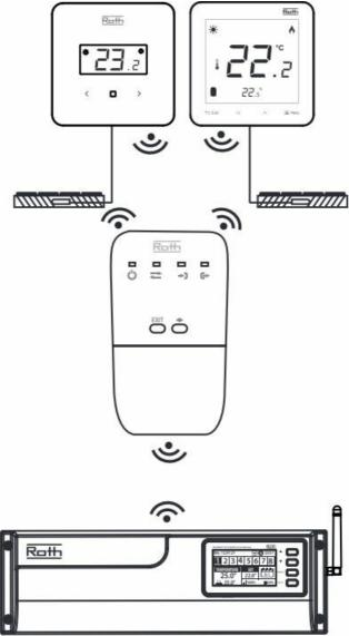
Connect the Repeater to the power supply – power indicator (A) will light up. Press the registration button (E) on the Repeater. The registration indicator out (D) will now be permantly on and the registration indicator in (C) will start flashing.
