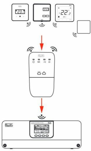
Connect the Repeater to the power supply – power indicator (A) will light up. Press the registration button (E) on the Repeater. The registration indicator out (D) will now be permantly on and the registration indicator in (C) will start fashing.) Press the registration button on the backside of the Room thermostat or Floor sensor. The registration indicator in (C) will now change to be permanently on and the registration indicator out (D) will start flashing.
