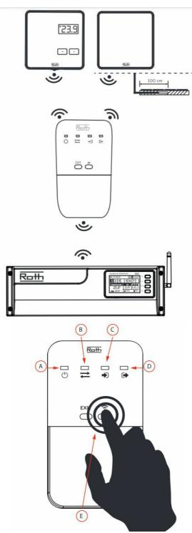
Press the registration button on the backside of the Room thermostat
