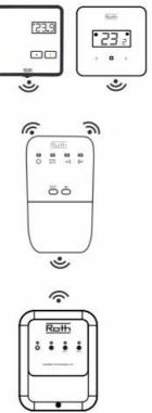
When the room thermostat is registered to the repeater, the repeater must be registered to the desired channel on the control unit, press once for channel 1 and twice for channel 2 on the registration button on the left side of the receiver. Check on the receiver that joints Ch.1 /Ch.2 turn on when the room thermostats call for heat.
