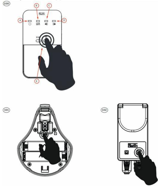
When the sensor is registered to the repeater, the repeater must be registered to the control unit. Press and hold the tick button for approx. 5 seconds until the LED starts flashing blue slowly. When the installation of the sensor via the repeater is completed, the LED will light blue for approx. 10 seconds.
