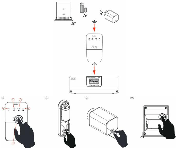
On the master, select "Windows sensor" or "Radiator actuators". You can connect up to 6 smart home devices per. channel. Select "Registration" and press "Yes" When the units have found each other, the LEDs on the repeater flash 5 times, after which the LEDs go out, with the exception of "Power".
