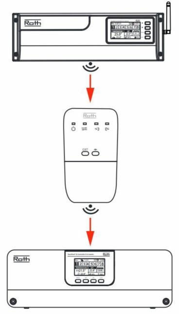
Registration and configuration of repeater between master and expansion module In a system, one may need a repeater between the master and one or more expansion modules. It is important to configure the master unit to the repeater before signing up for the expansion module, as this will ensure that all communication is properly exchanged between the two units.
