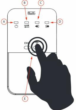
Press the registration button on the backside of the Room thermostat or Floor sensor. The registration indicator in (C) will now change to be permanently on and the registration indicator out (D) will start flashing.
