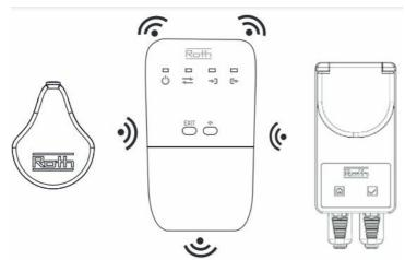
Press the registration button inside the sensor. The registration LED on the repeater "in" (C) will now light up constantly and the registration LED "out" (D) will flash.
