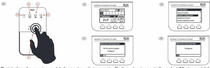
Registration of expansion module for master unit via repeater On the extension controller, select "Master module". Select "Registration" and press "Yes".
