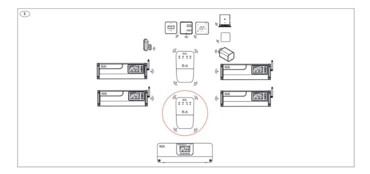
Connect the Repeater to the power supply – power indicator (A) will light up. Press the registration button (E) on the Repeater. The registration indicator out (D) will now be permantly on and the registration indicator in (C) will start flashing.
