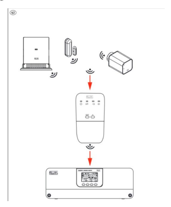
Setting up repeaters in between Smart Home components and master. First connect the repeater to 230V voltage, the power diode will light up (A). Press the register button (E). The registration LED "out" (D) will now light up constantly and the registration LED "in" (C) will flash. Press the registration button on the devices.
