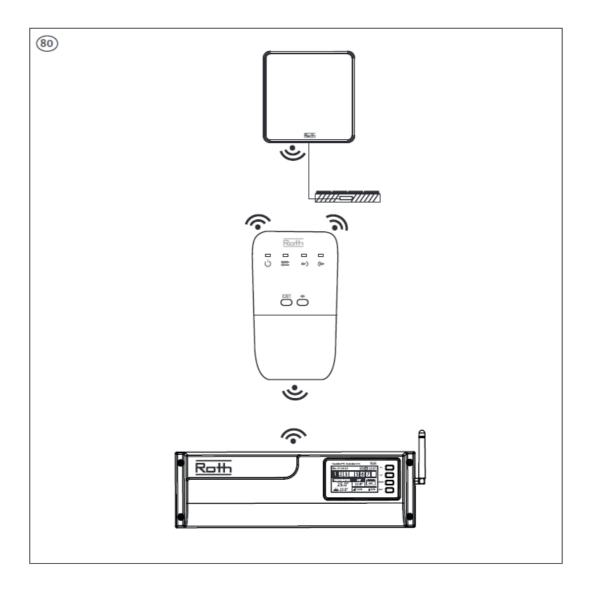
Press the registration button (E) on the Repeater. The registration indicator "out" (D) will now be permantly on and the registration indicator "in" (C) will start flashing
