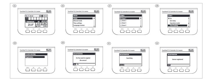
If installing a Floor sensor, follow the registration process on the Controller to register the Repeater to the zone.
