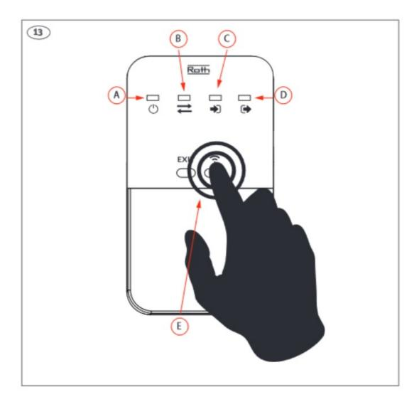
Connect the Repeater to the power supply – power indicator (A) will light up. Press the registration button (E) on the Repeater. The registration indicator out (D) will now be permantly on and the registration indicator in (C) will start flashing.
