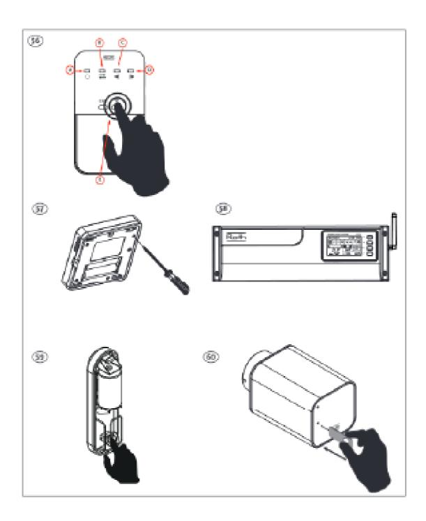
Setting up repeaters in series (56) Connect the first repeater to 230V voltage, the power diode will light up (A). Press the register button (E) on the repeater. The registration LED "out" (D) will now light up constantly and the registration LED "in" (C) will flash.
