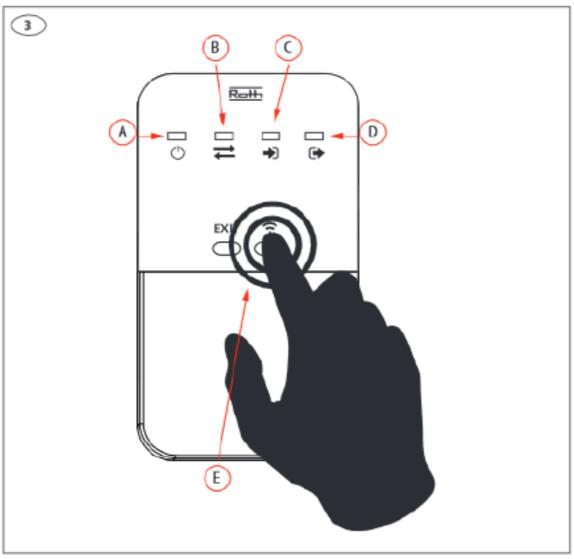
(UK) Press the registration button on the backside of the Room thermostat or Floor sensor. The registration indicator in (C) will now change to be permanently on and the registration indicator out (D) will start flashing.
