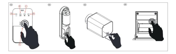
On the master, select "Windows sensor" or "Radiator actuators". You can connect up to 6 smart home devices per. channel. Select "Registration" and press "Yes" When the units have found each other, the LEDs on the repeater flash 5 times, after which the LEDs go out, with the exception of "Power".
