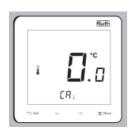
The room thermostat can show calibration value. Hold down "Me nu" for 3 sec. The display shows "Cal" and the calibrated temper ature. The value can ONLY be changed on the control unit, unde r the relevant channel/zone. It can take up to 5 minutes before the calibrated temperature is displayed.
