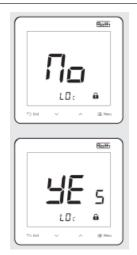
How to lock the buttons. Press "Menu" Select "Yes" using one of the  $\vee$  /  $\wedge$  buttons and confirm by pressing "Menu" or wait 5 seconds. When the lock is active, the keys are locked automatically af ter 10 seconds of inactivity. Unlock by pressing both  $\vee$  /  $\wedge$  buttons for 5 sec. The keys are available when the display does not show the lock. The lock is active until you deactivate it in the men u.
