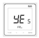
The room thermostat can be deleted from a control unit by pressing "Menu" for 3 sec., Release and briefly press "Menu" again. FA r is set to NO by default, to change this use " $\vee$  /  $\wedge$  ". At "Yes" press "Menu" or wait 5 sec and the thermostat is cleared from the control unit.
