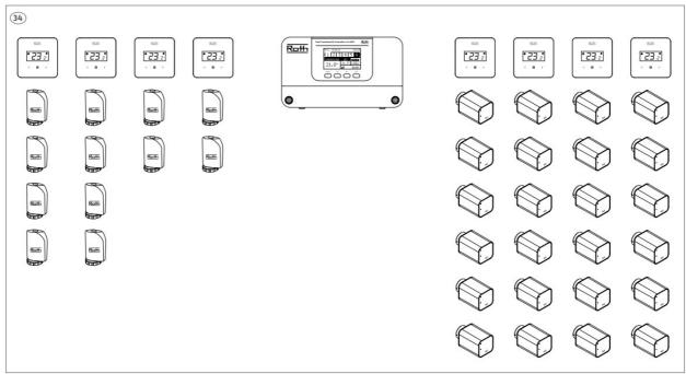
Registration of the actuator for the Roth Touchline® SL controller. Before you can register an actuator for a channel/zone, a thermostat must be registered, see the instructions for the thermostat.
