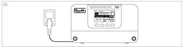
Connect to 230V power, Controller is ready for pairing of sensors. Follow the description later in this manual or please see the manual delivered with thermostat/sensor.
