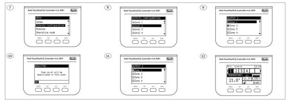
Press the MENU button on the controller and follow the steps 7 - 12. In this example output 2 is moved from zone 2 to zone 1.
