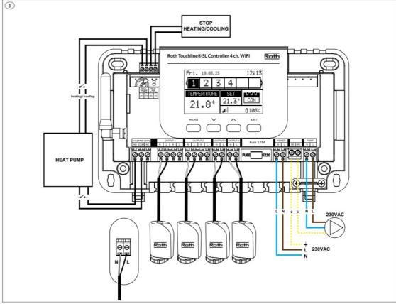
If required up to 4 actuators can be connected to output 1 og 2.
