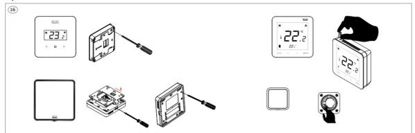
Above you can see the placement of pairing/registration button on different thermostats/sensors.
