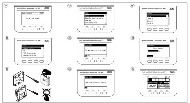
Follow the steps 17 – 25 for pairing/registering the thermostat/sensor to a zone/channel. Finish by pushing MENU button and push EXIT several times until start screen is shown.
