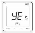
• The room thermostat can display the firmware version, by pressing "Menu" for 3 sec., Releasing and pressing twice briefly on "Menu.
