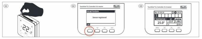
• Once the thermostat is connected to the Zone/Channel, the overview shows: – Temperatures on the thermostat (setpoint 22,0°C, actual 25,0°C). battery (99%), signal strength (appears with 4 lines, there must be a minimum of 1 line during installation), and mode of operation (CON = continuously). For more info on the display, see the
