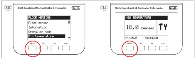
• Set min. floor temperature for your comfort level. Confirm with "Menu". Min. temperature is set as described above.
