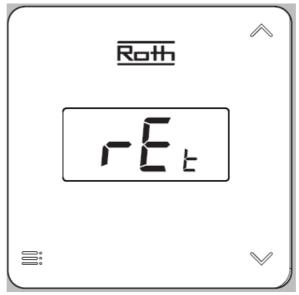
• Enables you to return from the MENU manually. After selecting "rEt" the screen flashes for 5 sec. and returns to view of the current temperature.
