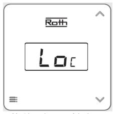
• Enables you to lock the buttons. Select "Yes" by using one of the buttons < >, confirm by pressing or wait 5 seconds. When the lock is active, the keys are locked automatically after 10 seconds of in-activity. To unlock, press and hold the bottoms < > for 10 sec. The keys are accessible when the display returns to showing the current temperature. The key lock is activated until you inactivate it in the menu.
