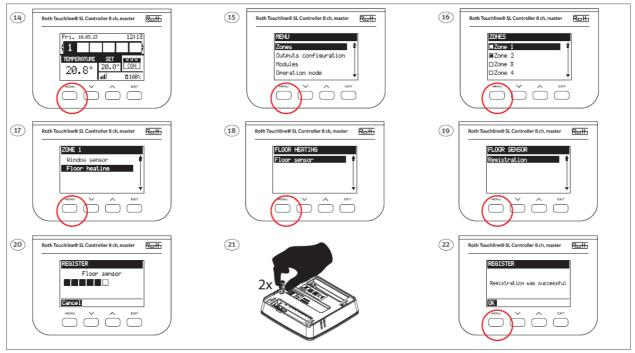
• If the thermostat has a floor sensor connected, this must also be paired/registered as shown below (picture 21, must be two quick presses).
