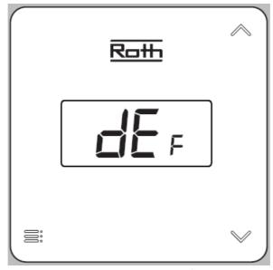
• Enables you to return the room thermostat to the factory setting. Select "dEF" and the display flashes and shows the selected value. Select/confirm (Yes) with < > buttons within 5 sec. Confirm by pressing or wait 5 sec. and the factory settings has be restored.
