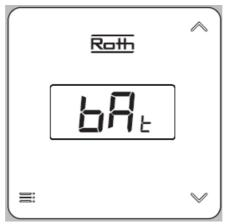
• Enables you to view battery level. Select "Bat", the display flashes. Confirm within 5 sec. after which the battery level is displayed in percentage %.
