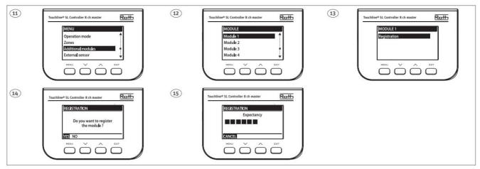
• When the devices have registered the connection, "OK" is displayed. Finish by pressing "Menu".
