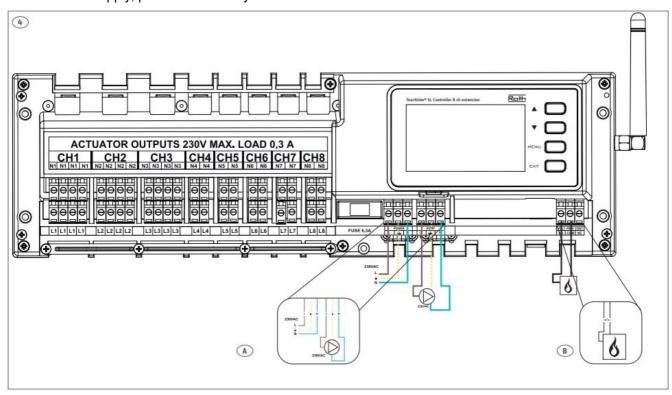
• Connect to 230V power, Controller is ready for pairing of sensors. Please see the thermostat/sensor operation manual.
