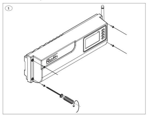
Must be mounted on a flat surface or using a DIN rail (not incl.), screws max. Ø 4 mm.
