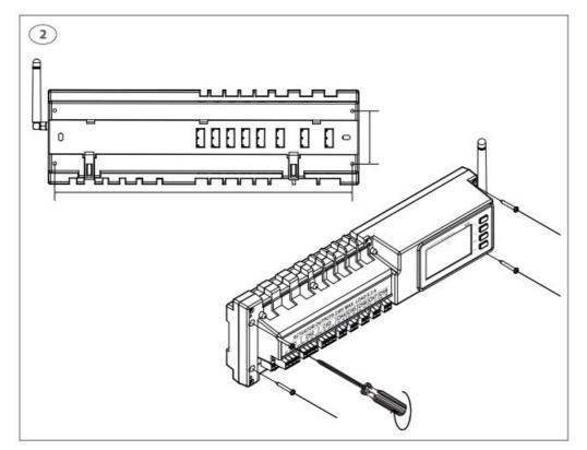
Actuators, connect "brown" to L and "blue" to N. Use Roth Touchline® actuator 230V 1 watt, HVAC no.
