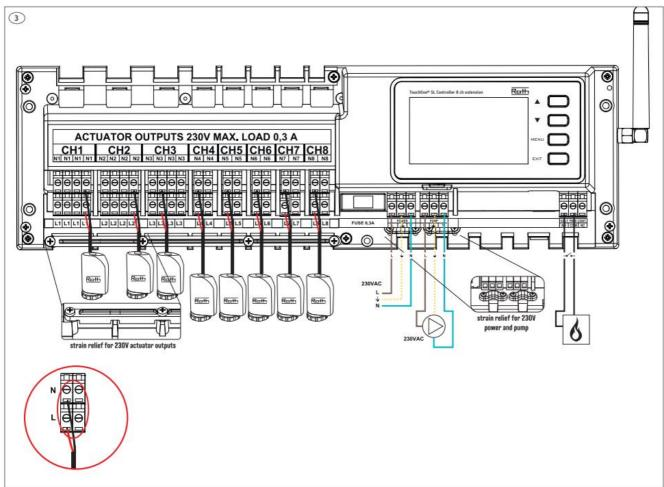
• A. 230V pump output, max. load 0,5A. Cables must be secured. The pump output on the control unit extension can either control a pump connected locally, or the signals (heat call from thermostats) can be set up to be
