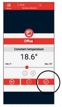
Used to bring the room back to normal operation. e.g. if this area should not be included in a time program or if the room is in "Party" mode.
