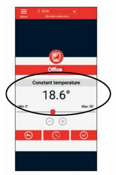
The desired temperature is set either by use of the +/- keys or the slider.
