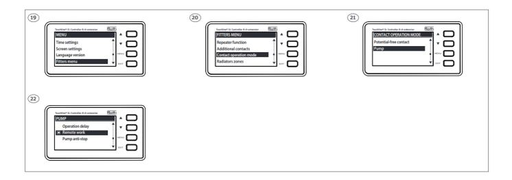
If the pump output is to be used to control the global pump connected to the control unit – master, the signal must be transmitted from the control unit – extension to the master control unit. Follow the steps on the screens for setting og the the control unit – extension.
