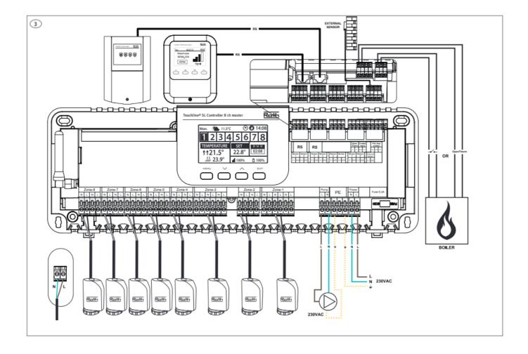
If required up to 4 actuator can be connected to the same output/ zone (32 actuators in total on the controller) Meaning: An output with 2, 3 or 4 terminals can all be connected with up to 4 actuators. Use Roth Touchline® actuator 230V 1 watt, HVAC no. 7466275433.
