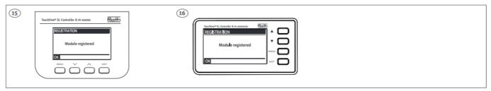
When the devices have registered the connection, "OK" is displayed. Finish by pressing "Menu".
