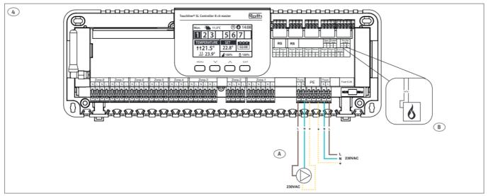
• 230V pump output, max. load 0,5A. Cables must be secured
