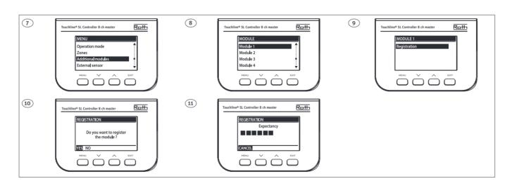
One Roth Touchline® SL Controller, master can be connected wireless with up to 4 Roth Touchline® SL Controllers, extension, meaning up to 40 channels in one system.
