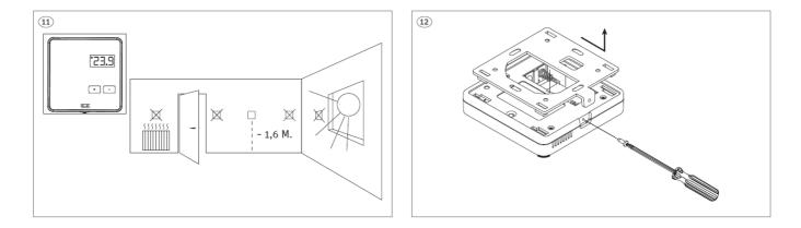
Remove screw and slide backplate off.
