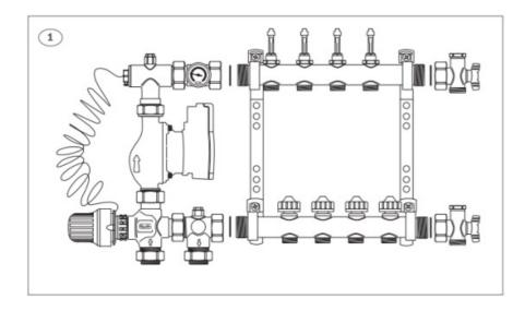
The shunt is mounted on the left, but it can be reversed by undoing all unions and rotating the pump.
