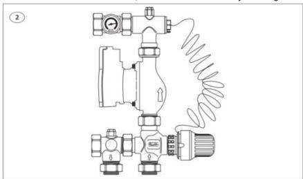
Mount the thermostat on the supply valve and the sensor in the sensor pocket. Set the thermostat to the preferred supply temperature. Lock the thermostat to an appropriate regulation range by pressing the white locking catches on the sensor element. See the scale in Figure 4.
