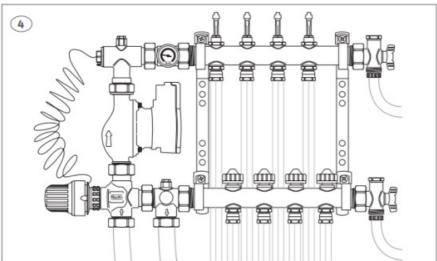
Venting and flushing the installation of air must be done one circuit at the time. Connect the filling hose to the upper manifold valve and the discharge hose from the lower manifold valve and flush to the drain. Refill the installation to desired pressure when all air has been removed.
