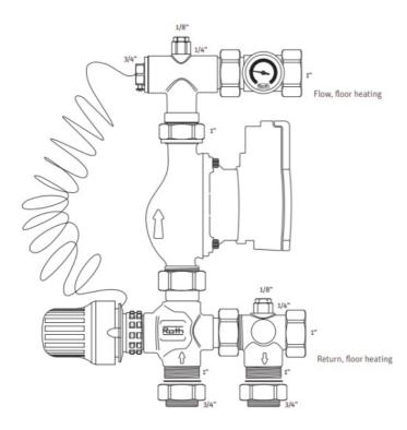
Roth shunt, 3-way valve: HVAC no. 7466210218
