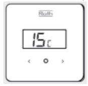
Enables you to adjust the hysteresis (tolerance of the preset temperature), which is preset to 0.2 K. Select "hYs" and the display flashes and shows the selected value. Select new value with < > buttons within S sec. Confirm by pressing • or wait 5 sec.
