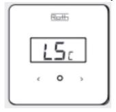
Enables you to adjust the hysteresis (tolerance of the preset temperature), which is preset to 0.2 K. Select "Lhy" and the display flashes and shows the selected value. Select new value with < ) buttons within 5 sec. Confirm by pressing • or wait 5 sec.
