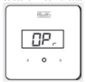
Enables you to return from the MENU manually. After selecting "rEt" the screen flashes for 5 sec. and returns to view of the current temperature.
