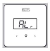
Enables you to adjust the calibration value. Select "ISc" and the display flashes and shows the selected value. Select new value with < buttons within 5 sec. Confirm by pressing • or wait 5 sec. Calibration range is from -10°C to +100C with the accuracy of 0.1°C.
