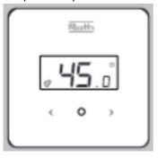
Enables you to view bat-tery level. Select "Bar, the display flashes. Confirm within 5 sec. after which the battery level is dis-played in percentage %.
