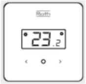
In sleep mode the current flow-temperature can be displayed. Press • to shift to flow-temperature. To set/change temperature press < > buttons. Confirm by pressing • or wait 5 sec.
