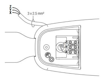
A switch or an omnipolar cut-off switch with a contact opening of at least 3 mm must be installed on the mains power line.
