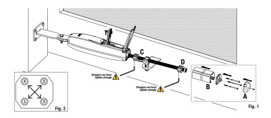
Use the internal mechanical stops in the piston as a supplementary safety measure in addition to the mechanical stops of the gate.
