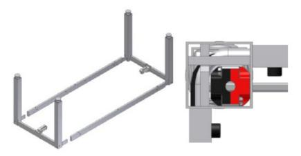
• Position the angle plate for control unit as shown and fasten it to front fascia.
