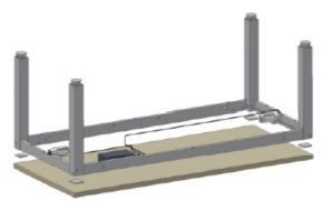
• Fasten the tabletop with screws through the holes of the fascias.
