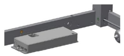
• Place the frame on the table top and push the cover plates between legs and table top. Centre the frame in relation to the table top.
