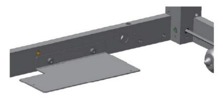
• Attach control unit to angle plate and fasten.
