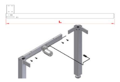
**Important:** Push side and front fascias firmly against the leg before retightening the fascias. Tighten the bolts securely by means of the wrench provided.
