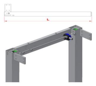
6.1.1 Check that the height (L) of all four legs is identical. May be adjusted on hexagonal shaft by means of the open-end wrench provided. Place side fascia's on a plane surface and mount legs. See label on legs.
