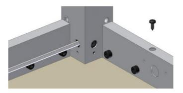
6.1.5 Fix the table top with screws through the holes of the fascia's.
