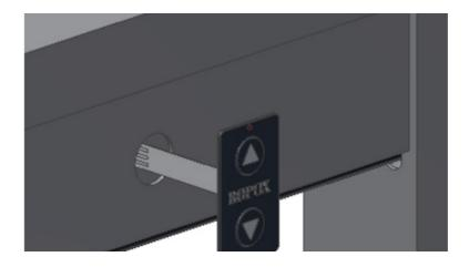
6.1.10 Mounting of fixed control switch Pull the cable through the front fascia and insert it into the control unit.
