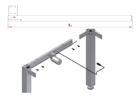
6.1.4 Check that the height (L) of all four legs is identical. May be adjusted on hexagonal shaft by means of the open-end wrench provided. Place side fascias on a plane surface and mount legs. See label on legs.
