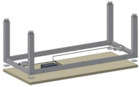
6.1.8 Place the frame on the table top and push the cover plates between legs and table top. Centre the frame in relation to the table top.
