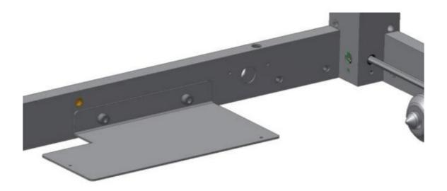
6.1.6 Position the angle plate for control unit as shown and fasten it to front fascia.
