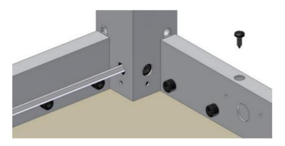
6.1.9 Fasten the tabletop with screws through the holes of the fascias.
