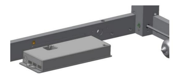
6.1.7 Attach control unit to angle plate and fasten.
