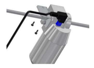
6.1.1 Mount hexagonal shaft and motor cable.
