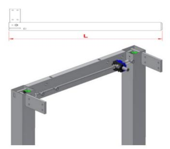
6.1.1 Check that the height (L) of all four legs is identical. May be adjusted on hexagonal shaft by means of the open-end wrench provided. Place side fascias on a plane surface and mount legs. See label on legs.
