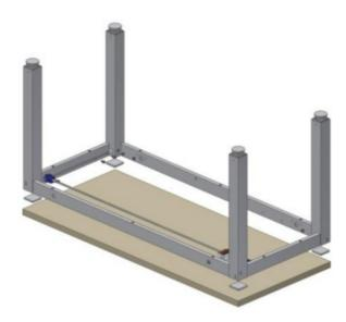
6.1.4 Place the frame on the table top and push the cover plates between legs and table top. Centre the frame in relation to the table top.
