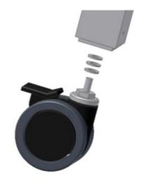
6.2.1 Mount the wheels. Do not forget to fit three washers on each wheel.
