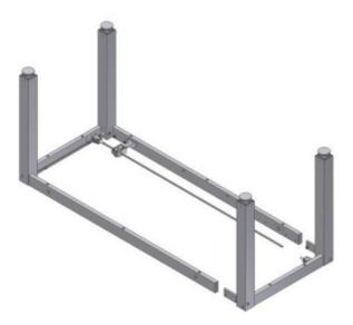
6.1.3 Now mount the two front fascias. Tighten the bolts securely by means of the wrench provided.
