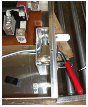
You must start with the top turnbuckle screw (attached to the switch movable) flush with the inside of the turnbuckle body.
