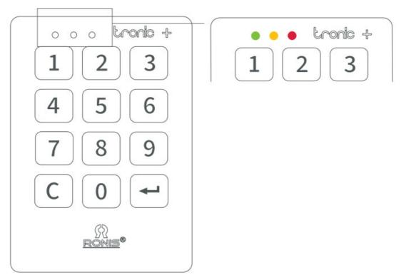
Dead or almost dead batteries: replace batteries.
