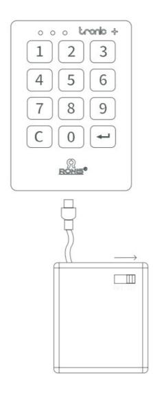
1. Make sure the battery pack contfull powered batteries (don't screw the battery pack too tight to avoid breaking the mechanism)
