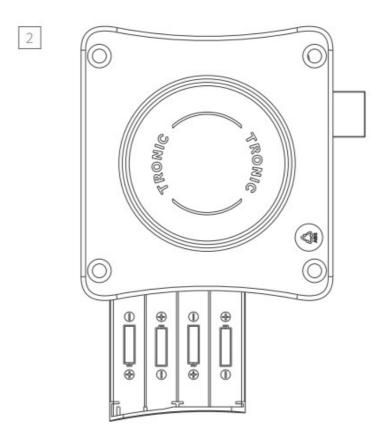
Relase the batteries thanks to T20 Torx Security screw located on the opposite of the battery case Verify that the batteries are in the right polarity (as indicated in the battery box).
