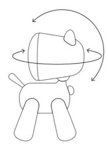
LED Lamp has rotatable construction. Before using, you can set the comfortable angle of light – just rotate the top part of device and fix the position.
