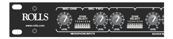
Each input is assigned to a Zone via the four DIP switches nearest that Input Level control. The zone is assigned when the switch is in the DOWN position. For example, the switch settings above send Mic 1 to all four Zones; 1, 2, 3, and 4. Mic 2 is sent to Zone 1 only. Source 1 is sent to Zone 1, and Source 2 is sent to Zones 2, 3, and 4.
