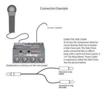
The plug connected to the Tip is the "Send" which will connect to the Input of the signal processing device, and the Ring is the "Return" which connects directly to the detector (compression control) circuit.
