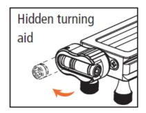
Loosen the panoramic locking knob [7] to be able to rotate the quick-release plate [3] 360°.
