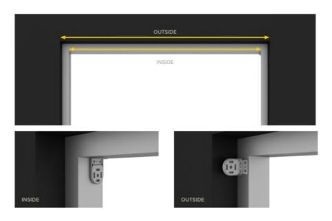
Place your first bracket in its mounting location and mark the screw holes. Place your second bracket in its mounting location and repeat the process.
