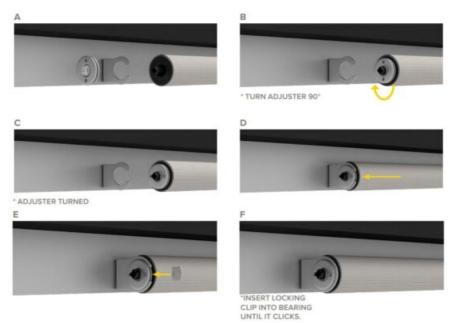
NOTE: Bearing clip cannot not be removed once engaged.
