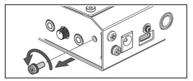
2. Using the screw that you removed in step 1, attach the cord hook as shown in the illustration.
