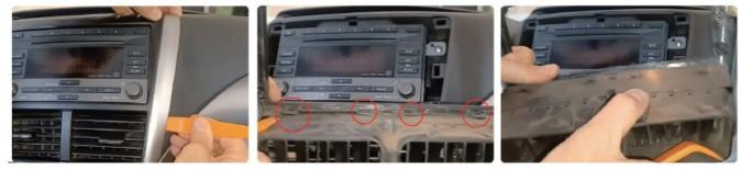
2. Use a screwdriver to unscrew the 4 screws securing the radio on both sides and remove the radio. Disconnect the cables between the radio and the original car.
